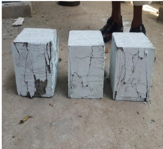
Figure 2. Cubes after testing
